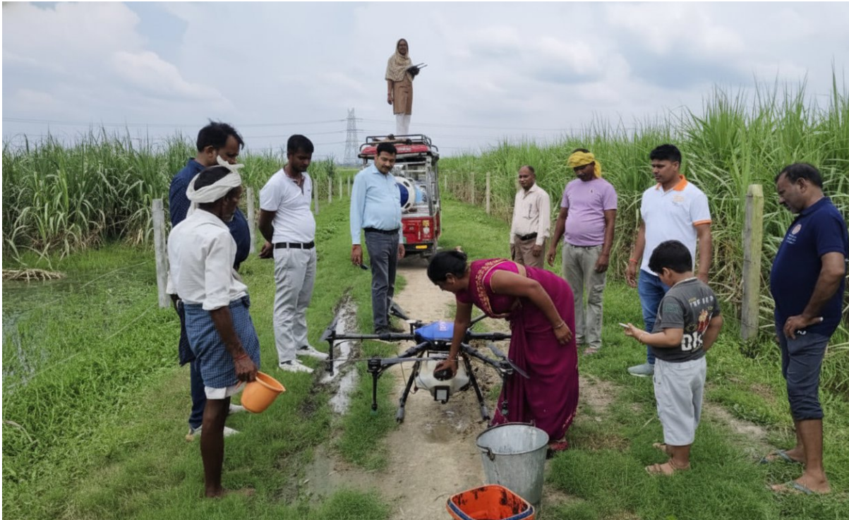
Picture 3 & 4: Ms. Shabiba Demonstrating pesticides application in dense canopy crop like in sugarcane and banana
