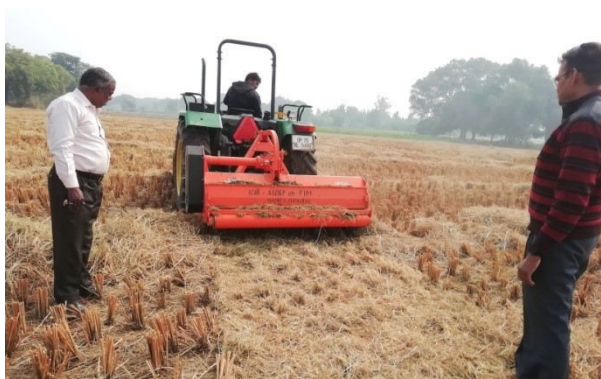
Paddy residues in-situ mulching by mulcher under CRM: KVK Prayagraj
