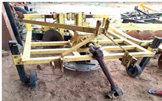
Tractor Drawn Ratoon Manager Machine traditional
